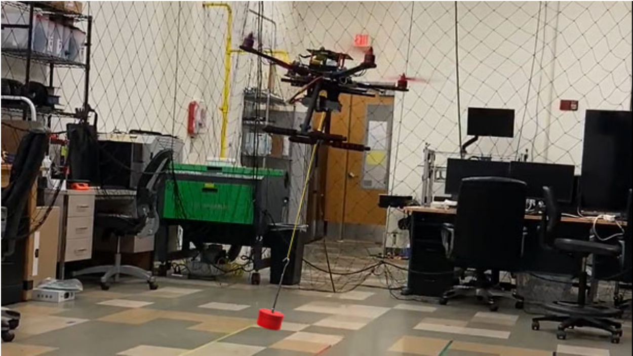
Figure 1: Experimental scenario: Carrying a load while trajectory tracking. The colors of the photo is edited to highlight the rope and the load.
