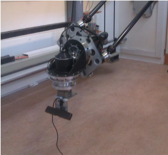
Fig. 10. L2 Gantry Tau Robot with mounted Xtion Asus Pro Live RGB-D camera.
